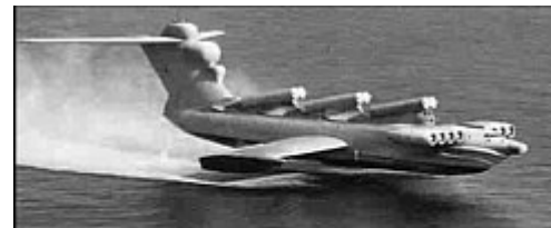
Ekranooplan with 6 guided missile tubes for "under the radar" hi-speed (250+ kts) attack and escape without detection
